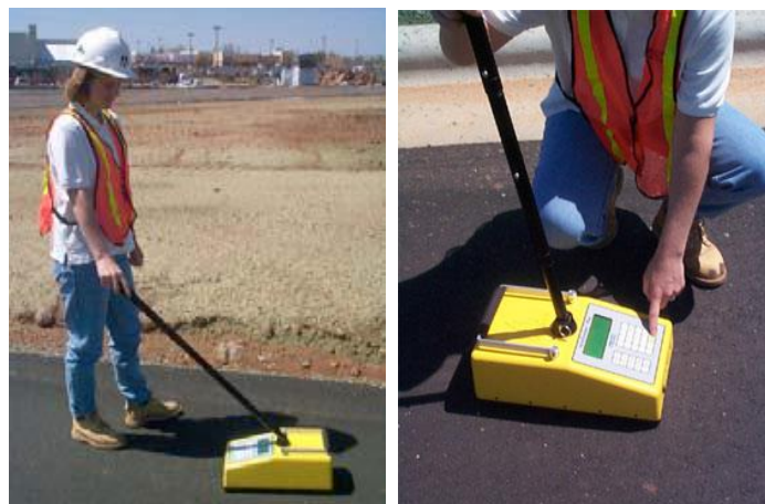
Figure 7 Model 2701B PaveTracker Plus by Troxler ( http://www.troxlerlabs.com/Portals/0/Troxler%20Documents/Marketing%20Documents/PaveTracker%202701-B/2701BSS102015.pdf )
