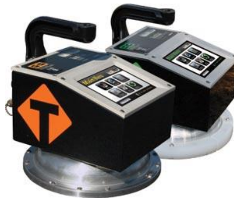
Figure 6 Model 380 PQI by TransTech ( http://www.transtechsys.com/products/index.php )
