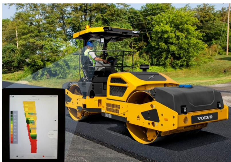
Figure 16 Intelligent Compaction System by Volvo (2015)
