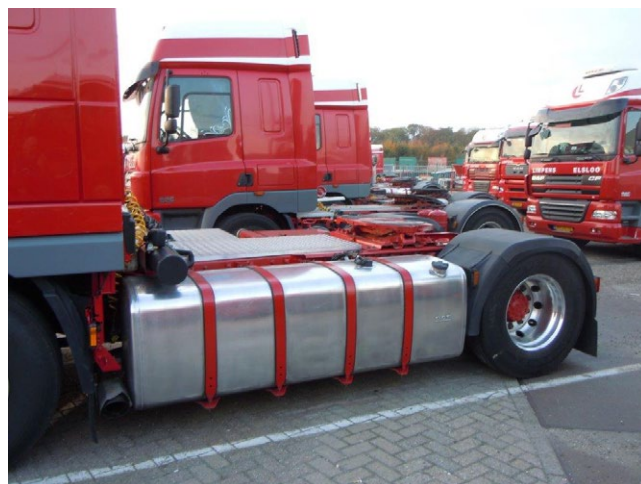
Positioning of guard rails on articulated vehicle (not protecting the fuel tank)
