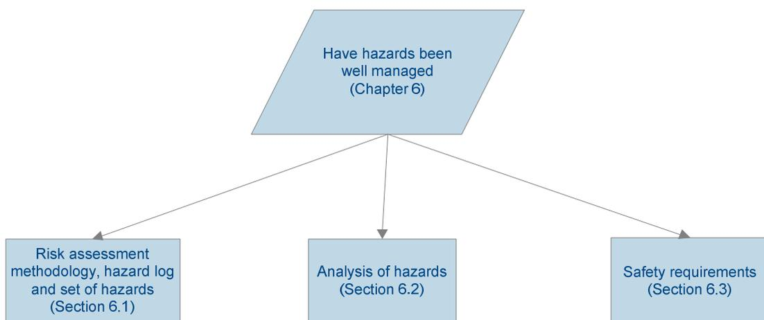
**Figure 6-1: Extract of GSN diagram showing how it is demonstrated that hazards have been well managed**
