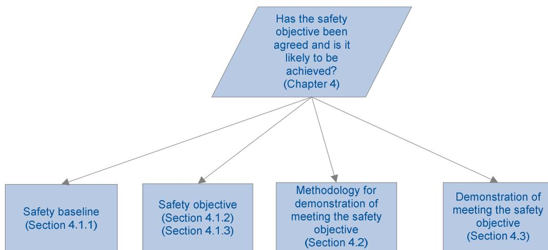
**Figure 4-1: Extract of GSN diagram showing how it is demonstrated that a safety objective has been agreed and is likely to be achieved**
