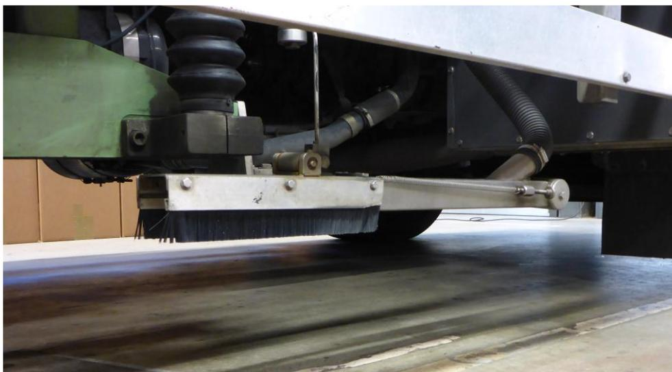
**Figure 4.2 Pavement wetting system on a SKM (raised position)**
