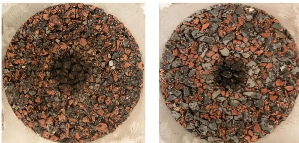
**Figure 4.4 Asphalt specimens containing a red aggregate in the 6/14 mm fraction (left) and in the 4/10 mm fraction (right)**
