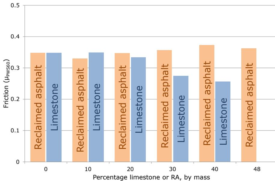
**Figure 4.5 Friction measured on asphalt specimens containing either limestone or RA in different proportions**
