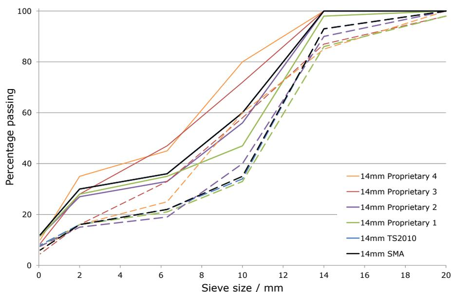
**Figure 3.2 Grading envelopes for 14 mm thin surface course systems**
