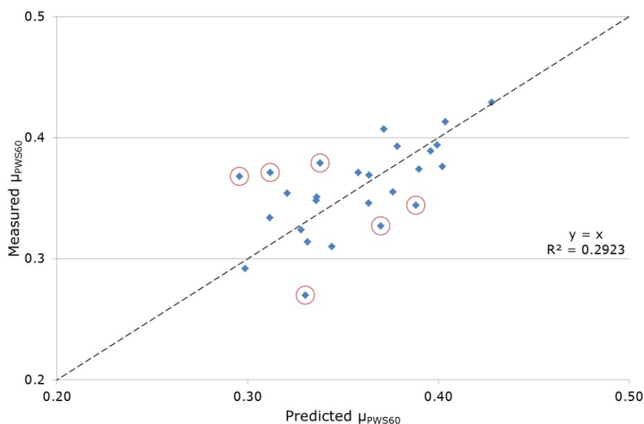
**Figure 4.3 Measured friction vs friction predicted using a regression formula**
