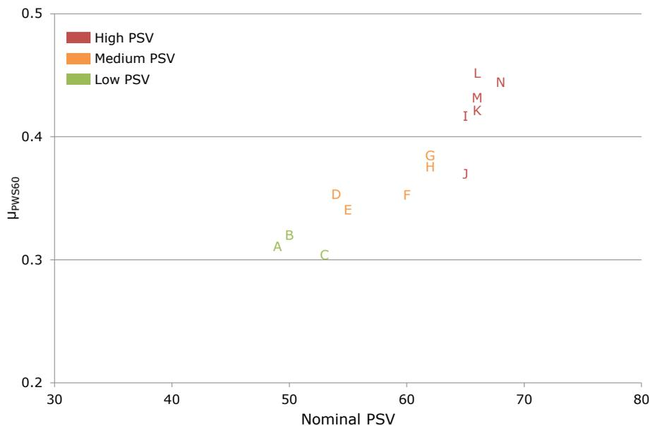
**Figure 4.1 Friction measured using the W-S machine against nominal PSV**
