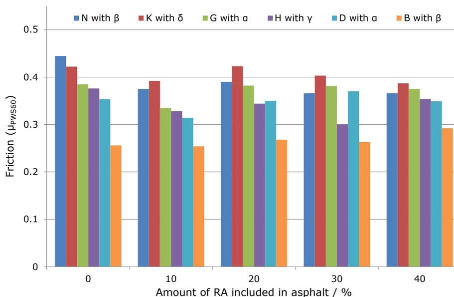
**Figure 4.6 Friction measured on asphalt specimens containing RA in different proportions**
