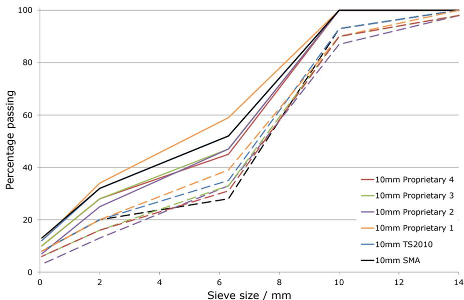
**Figure 3.1 Grading envelopes for 10mm thin surface course systems**
