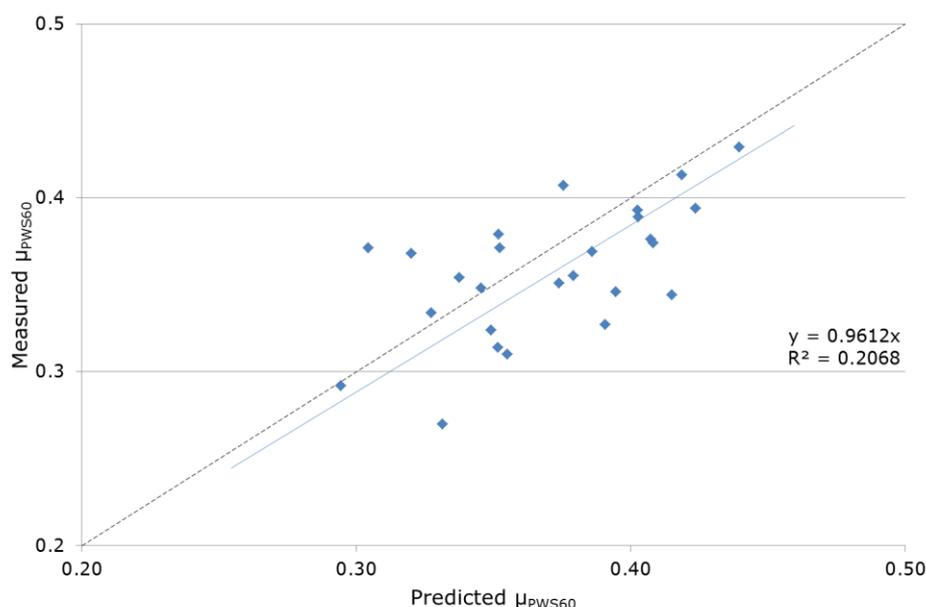
**Figure 4.2 Measured friction vs friction predicted using a mass ratio formula**
