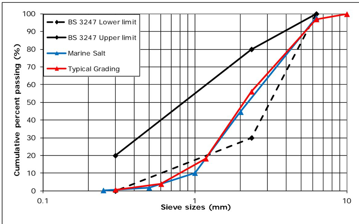
Figure 2. Grading of 8mm marine salt in accordance with BS 3247
