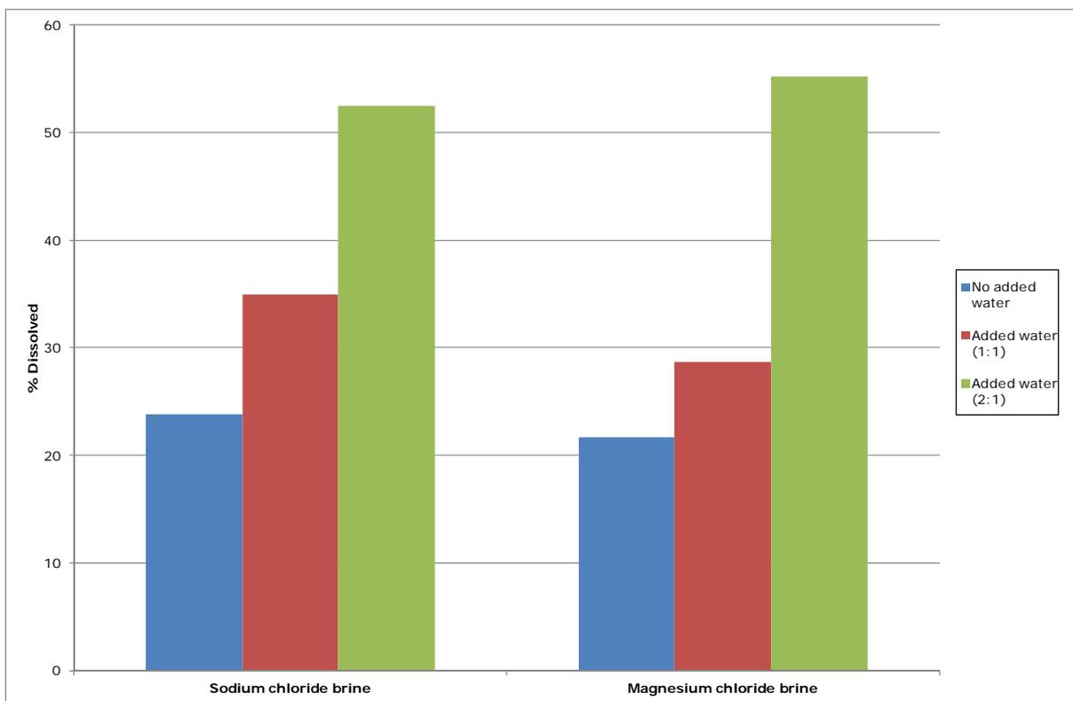
Figure 15. Comparison of salt dissolved at 0°C for 2 hours
