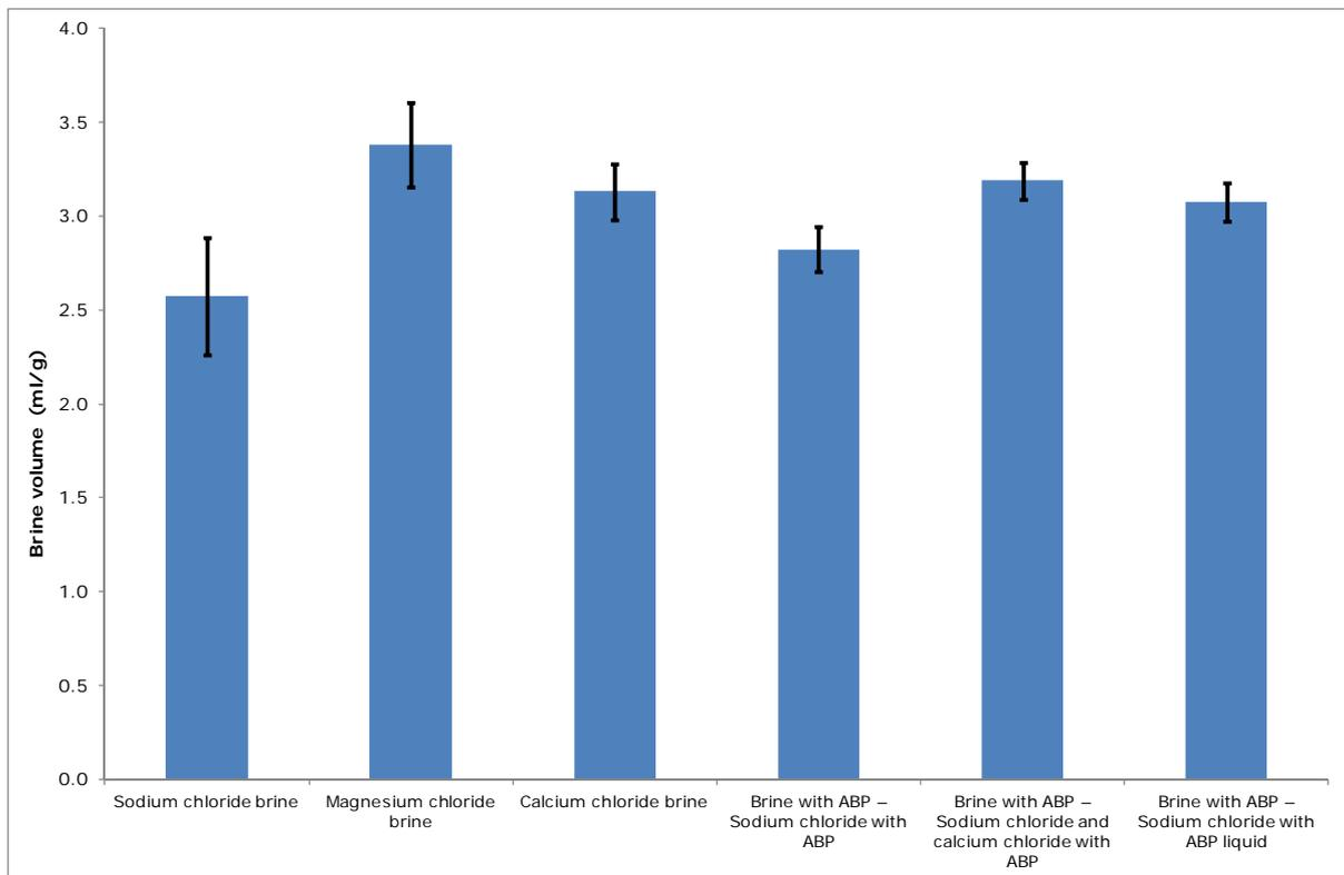
Figure 9. Comparison of the ice melting of pre-wetted rock salt at -12°C for two hours
