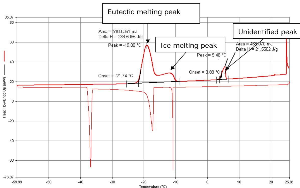
**Figure 16. DSC scan, 2°C per min, 10mg sample, Sodium chloride solution (20% de-icer)**
