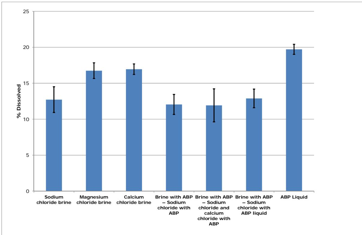
Figure 13. Comparison of salt dissolved at -12°C for two hours
