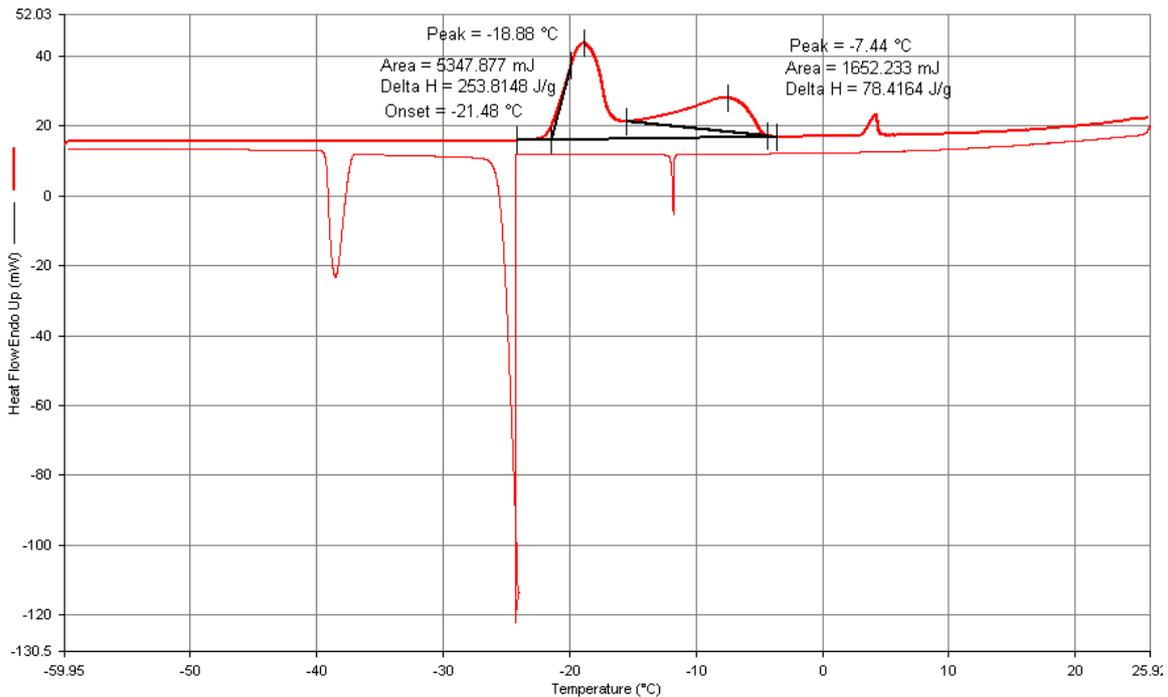
**Figure 17. DSC scan of 10 mg of sodium chloride solution at a rate of 2°C per min**
