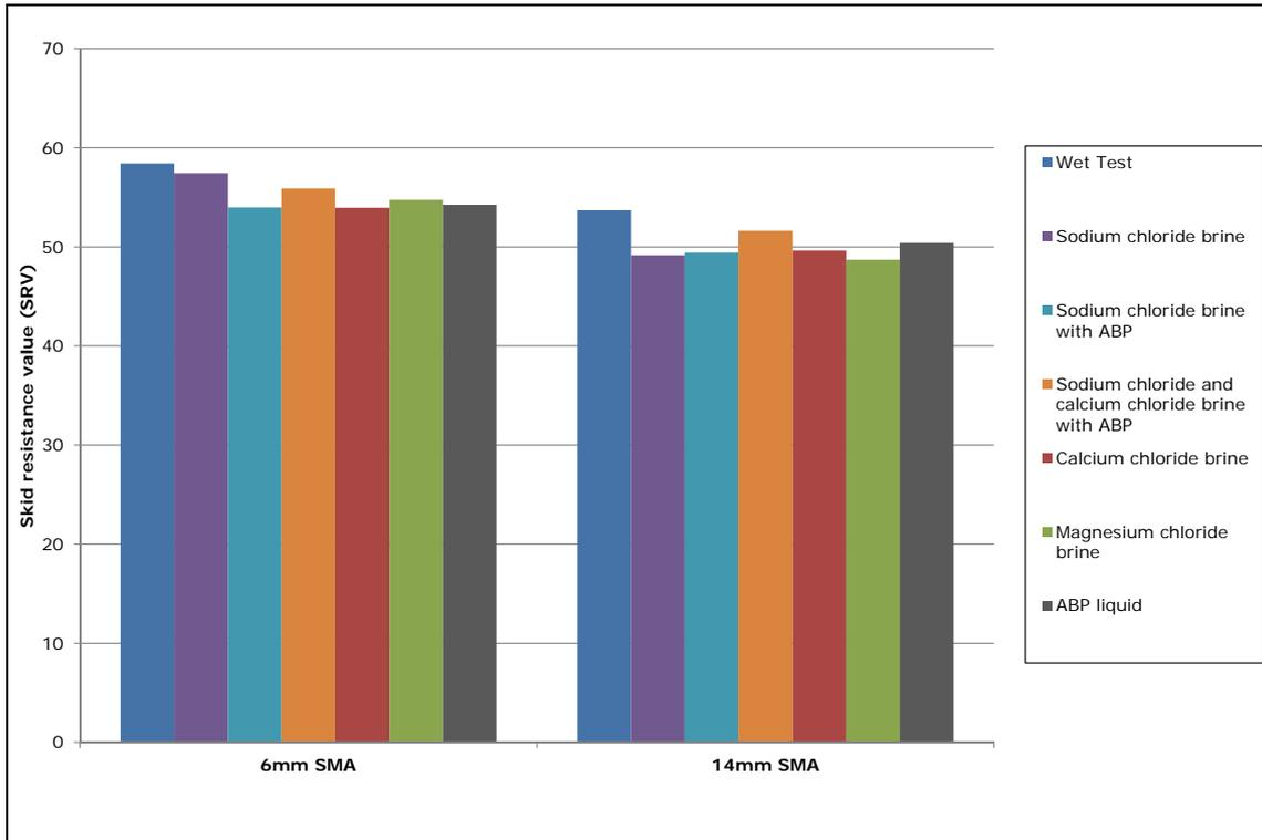
**Figure 25. Comparison of Skid Resistance Values (SRV) for 25% de-icer solutions**
