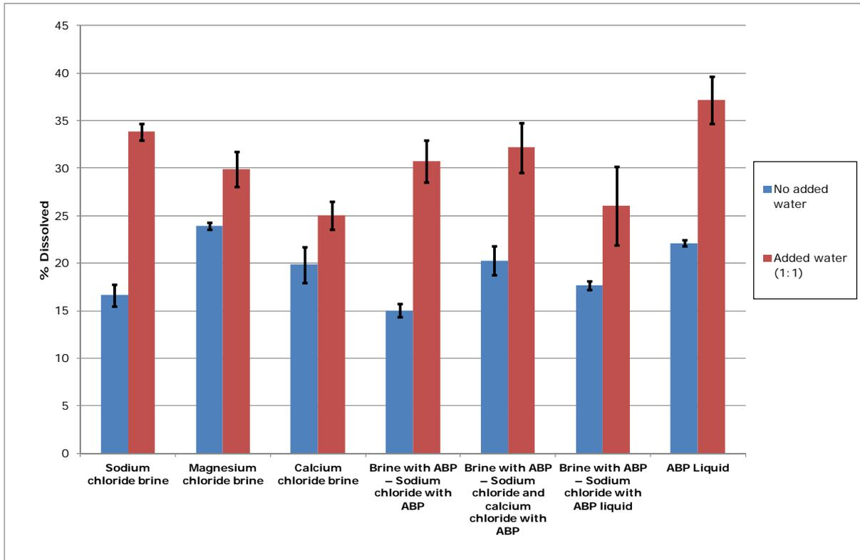
Figure 14. Comparison of salt dissolved with and without adding water, at -7°C for two hours
