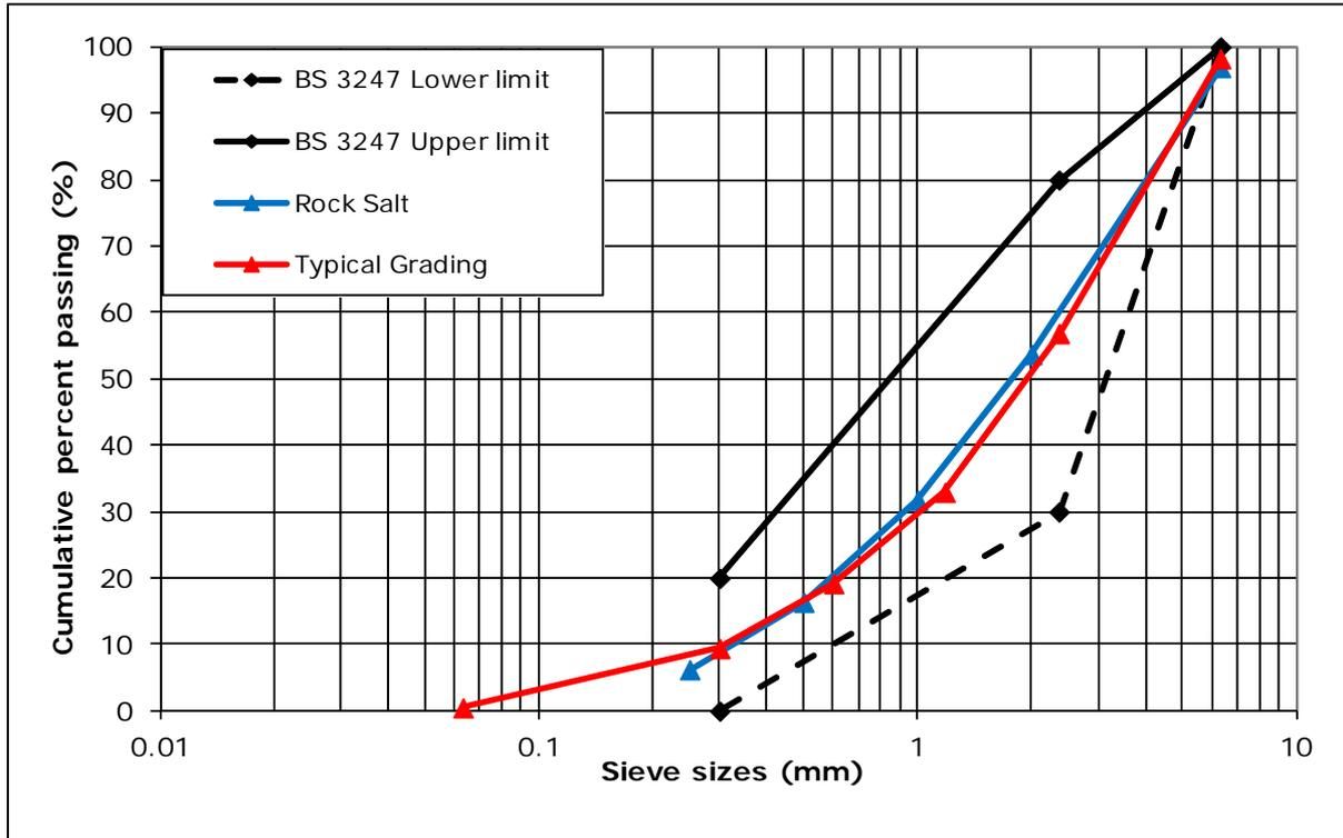
Figure 1. Grading of 6.3mm rock salt grading in accordance with BS 3247
