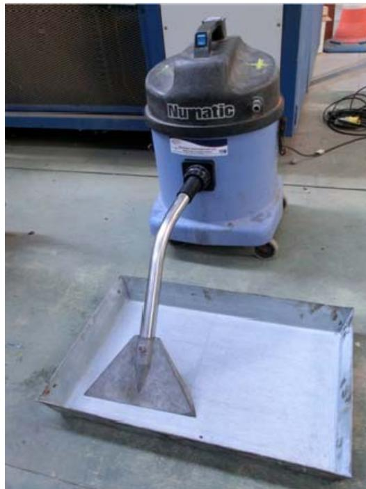
**Figure 10. Modified vacuum equipment**
