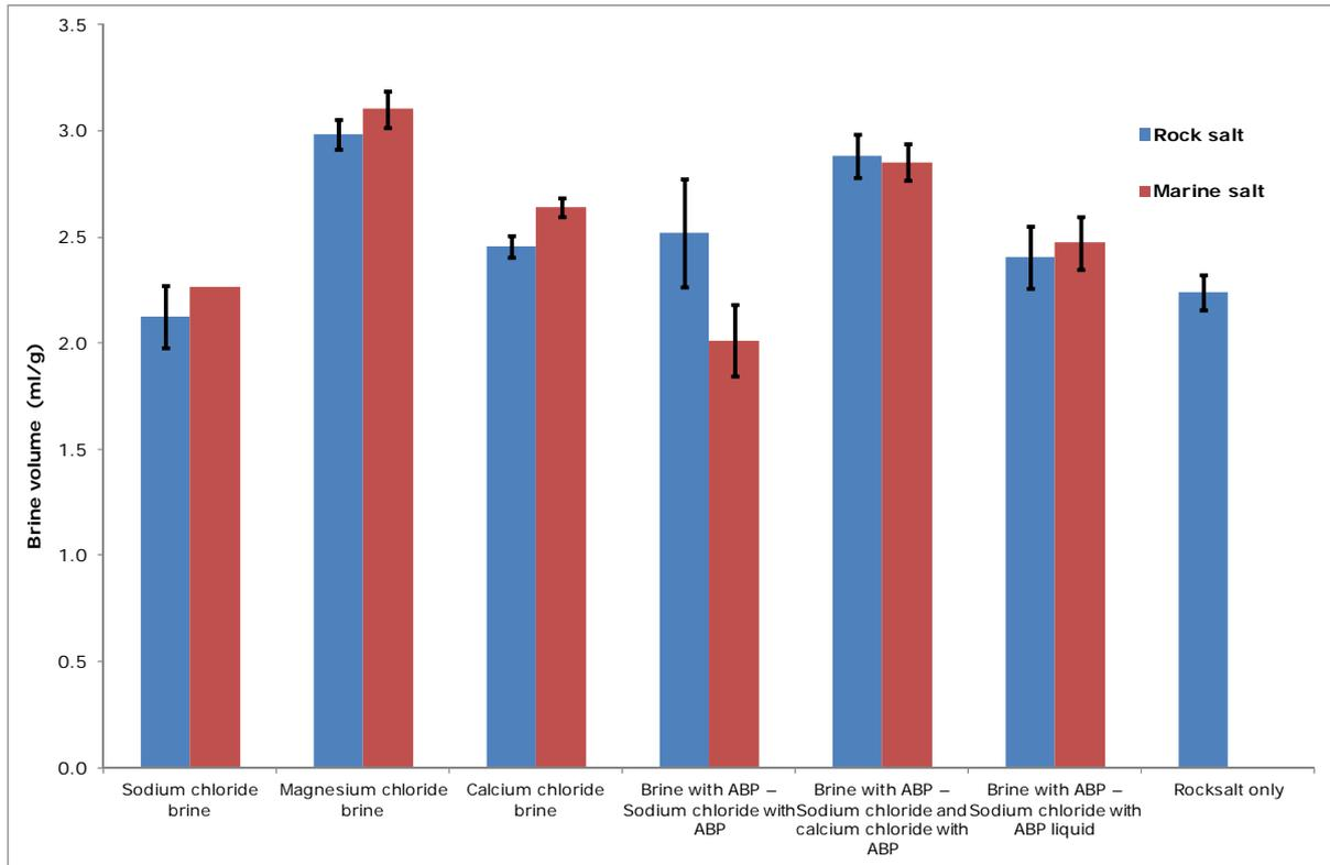
Figure 8. Comparison of the ice melting at -12°C for one hour
