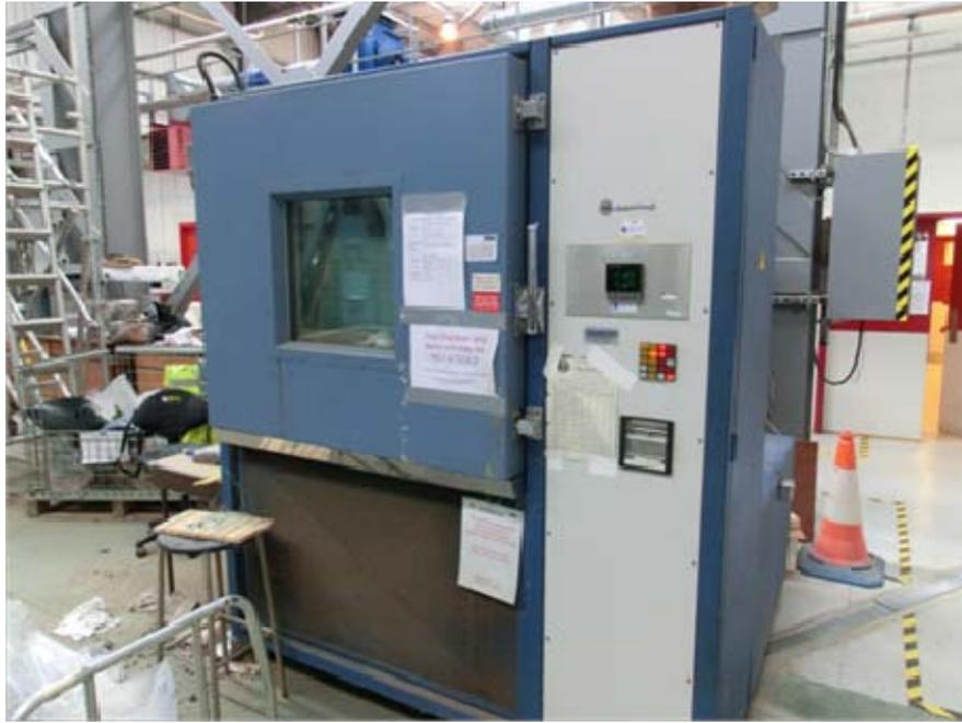
**Figure 4. Environmental test chamber**
