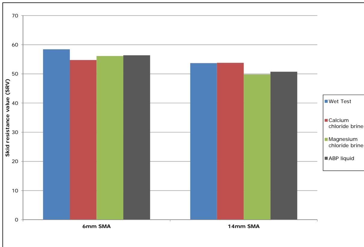
**Figure 24. Comparison of Skid Resistance Values (SRV) for diluted 1:1 de-icer solutions**
