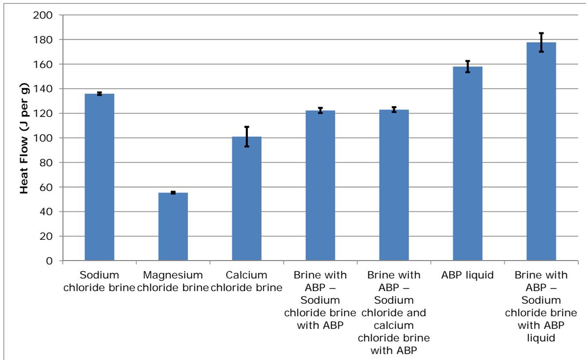
**Figure 22. DSC heat flow – diluted liquid de-icers**
