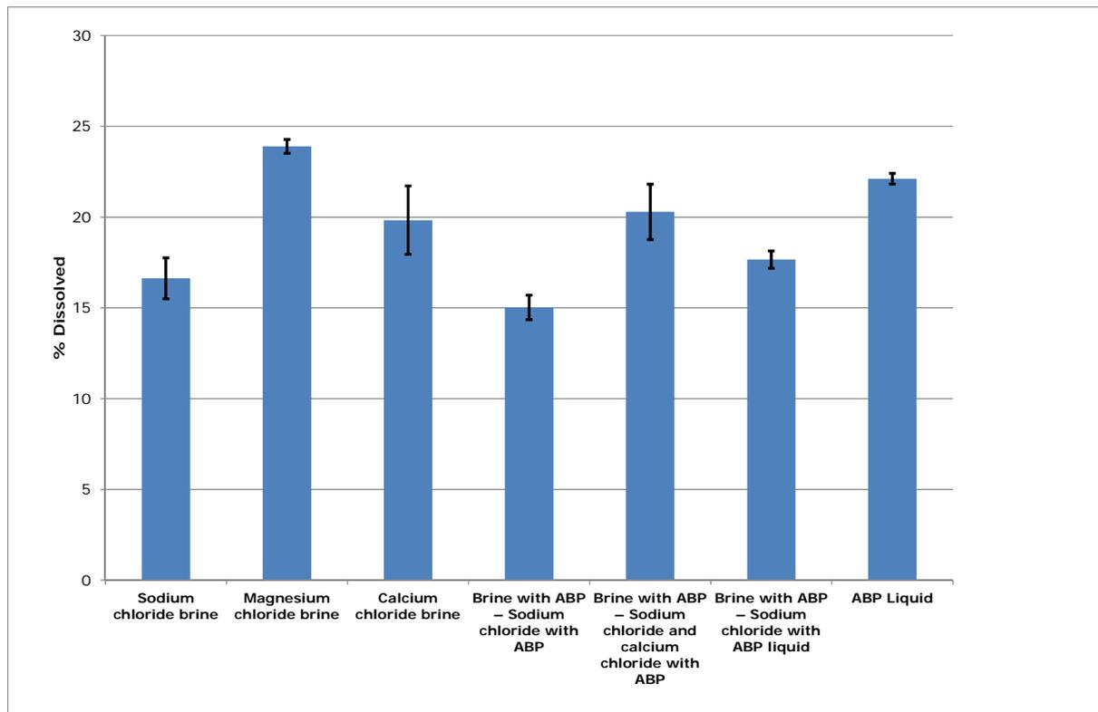
**Figure 11. Comparison of salt dissolved at  $-7^{\circ}\text{C}$  for 2 hours**
