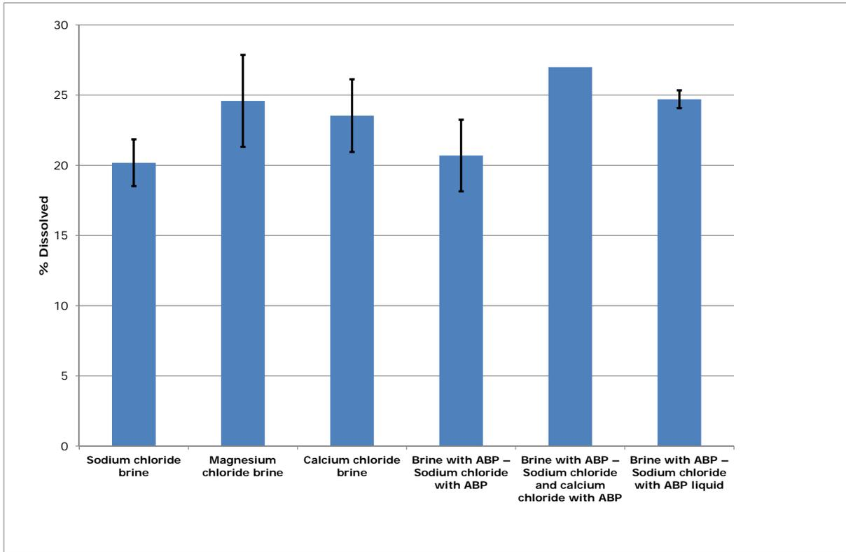
Figure 12. Comparison of salt dissolved at -7°C for 4 hours
