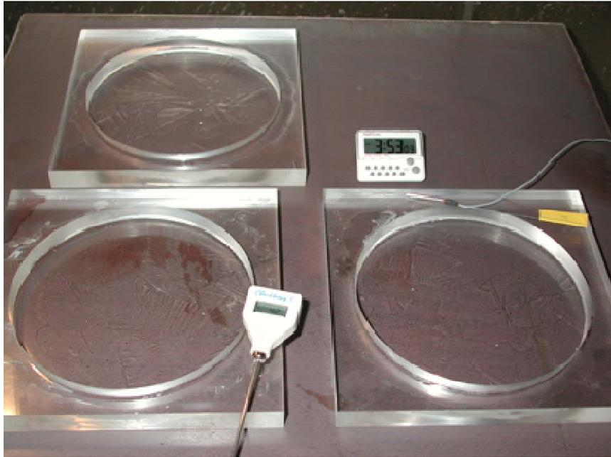
**Figure 3. 9 inch diameter ice samples in Perspex dishes**
