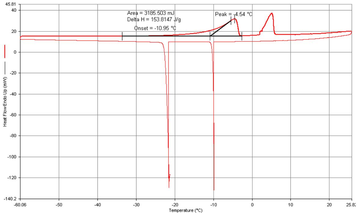
**Figure 18. DSC of 10mg of ABP liquid (40% solution)**
