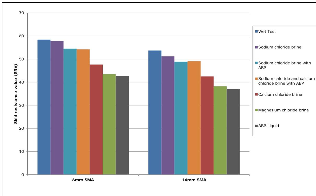
**Figure 23. Comparison of Skid Resistance Values (SRV) for liquids as supplied (not diluted in solution)**
