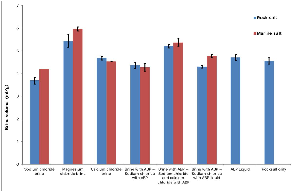
Figure 6. Comparison of the ice melting at -7°C for one hour
