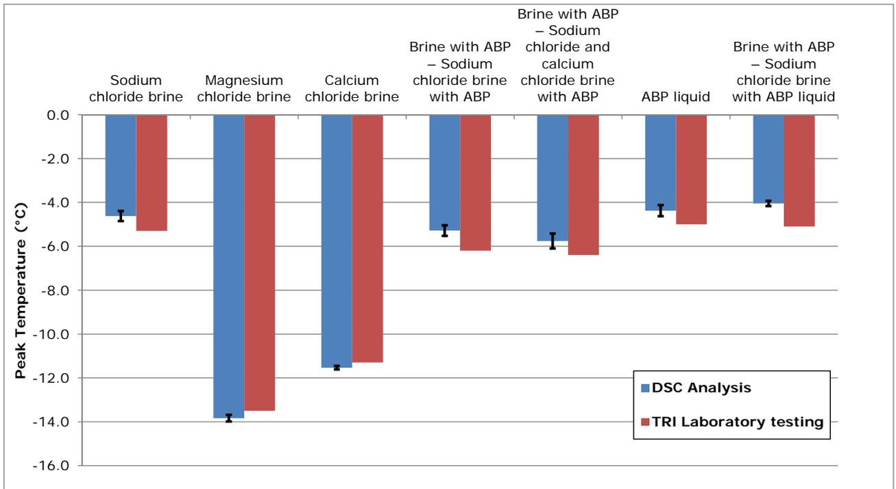
Figure 20. DSC Peak Temperatures diluted liquid de-icers
