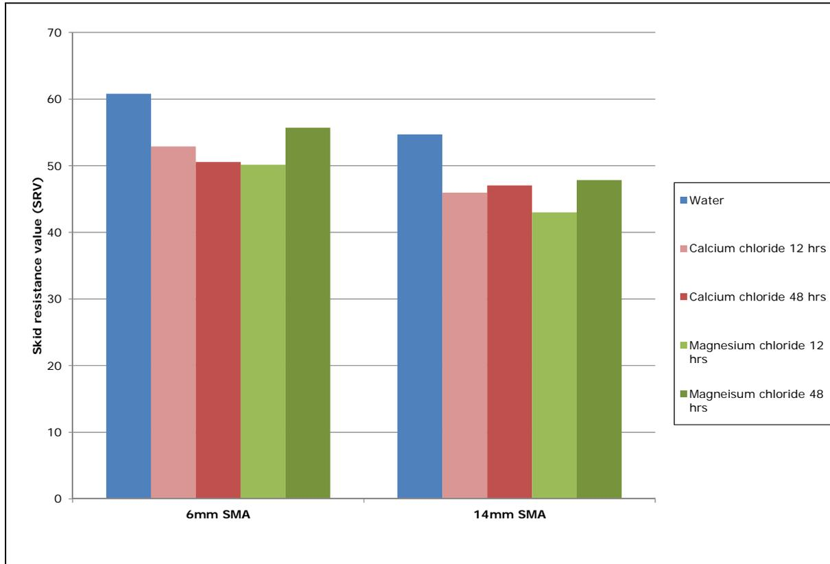
**Figure 26. Comparison of Skid Resistance Values (SRV) for de-icer solutions**
