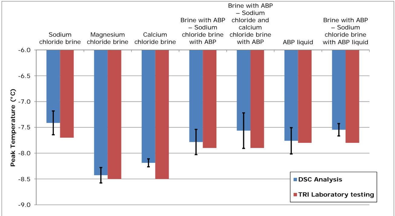
Figure 19. DSC peak temperatures for 15% de-icer solutions
