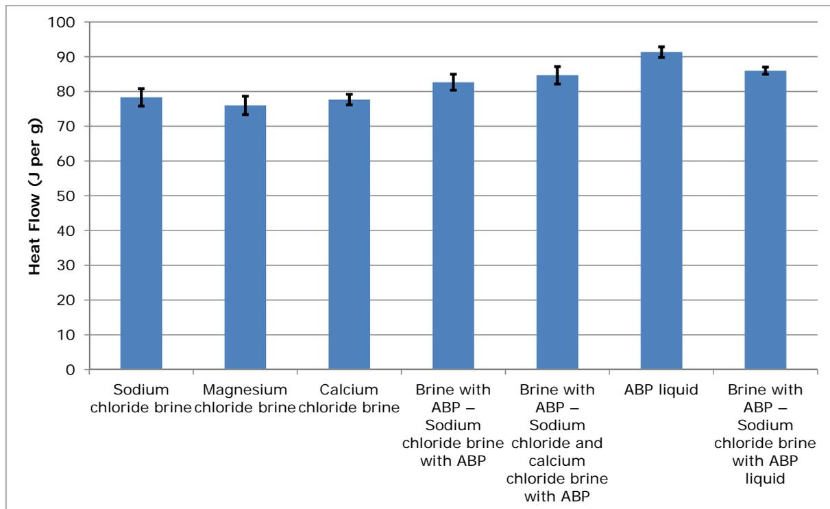
Figure 21. DSC heat flow – 15% de-icer solutions
