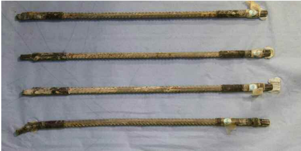
Figure 24: Top surface of bars removed from Specimen 8A
