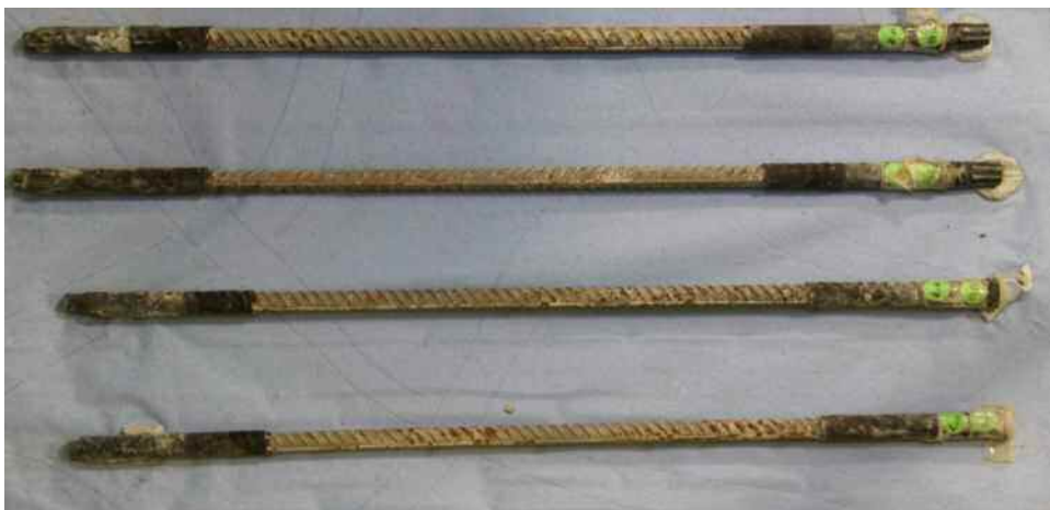
Figure 29: Top surface of bars removed from Specimen 22A
