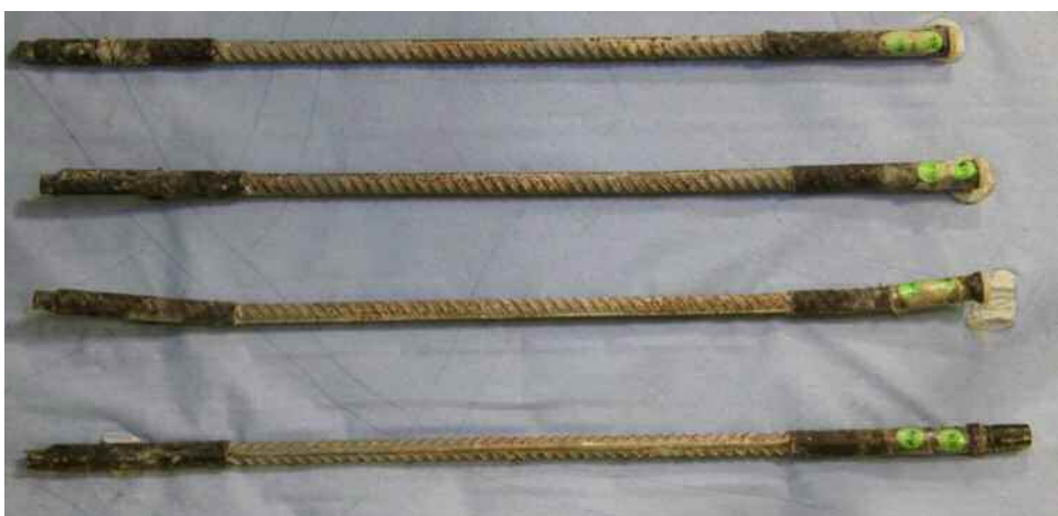
Figure 26: Top surface of bars removed from Specimen 15A
