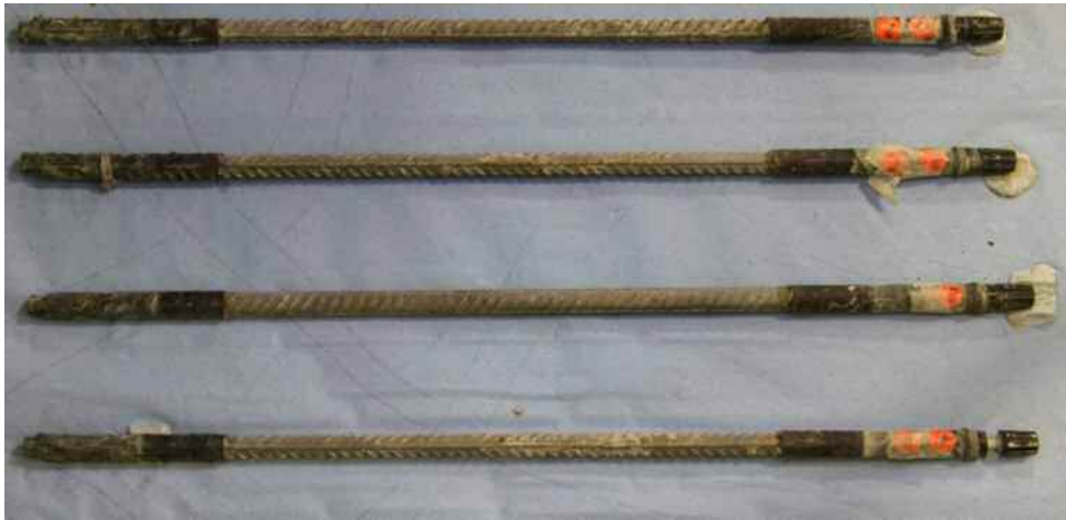
Figure 28: Top surface of bars removed from Specimen 20A
