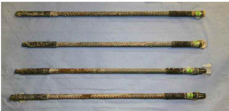
Figure 23: Top surface of bars removed from Specimen 6A
