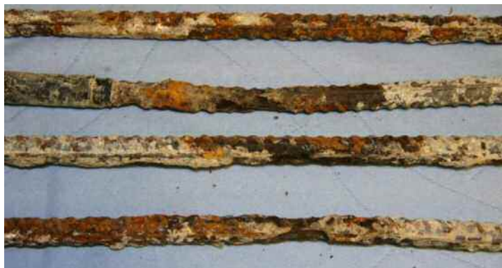
Figure 15: Close up photograph of bars removed from the specimens containing Lightweight Aggregate B
