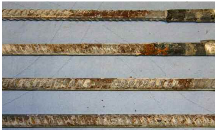
Figure 14: Close up photograph of bars removed from the specimens containing Lightweight Aggregate A
