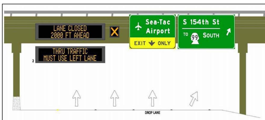
**Figure 9: Example Layout of Junction Control System**
