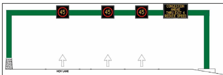
**Figure 7: Example Layout of a Speed Harmonisation System**
