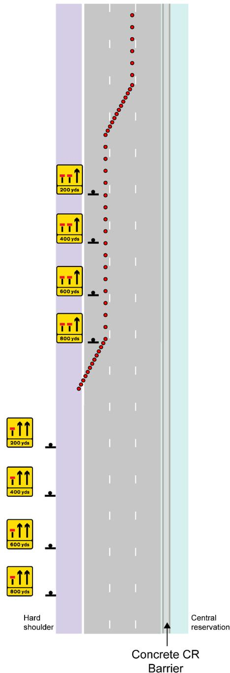
**Figure 8: Additional idea for TTM on motorways with concrete barrier**
