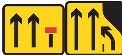
**Figure 1: "Wicket board" and "hooked arrow" lane closure signs**
