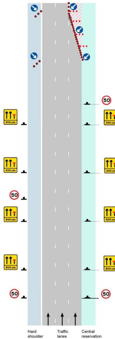
**Figure 4: Proposed closure layout control – Current Chapter 8 layout**
