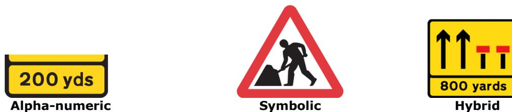
**Figure 2: Different forms of signage that are in use at road works**
