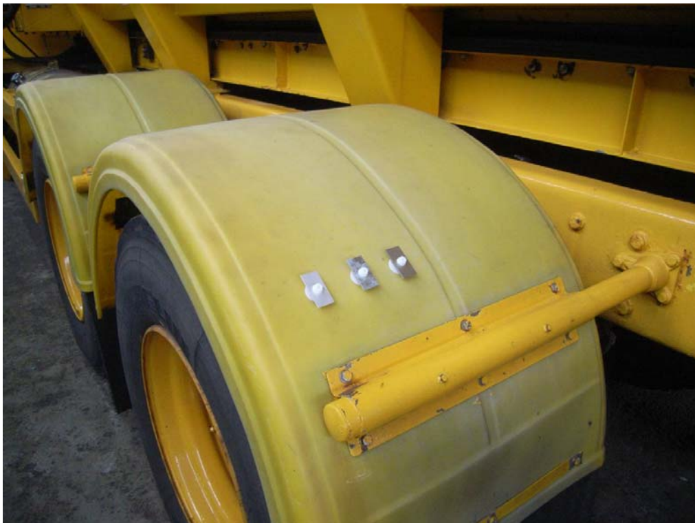
Plate 2-4 Polyethylene mudguard on Foden vehicle
