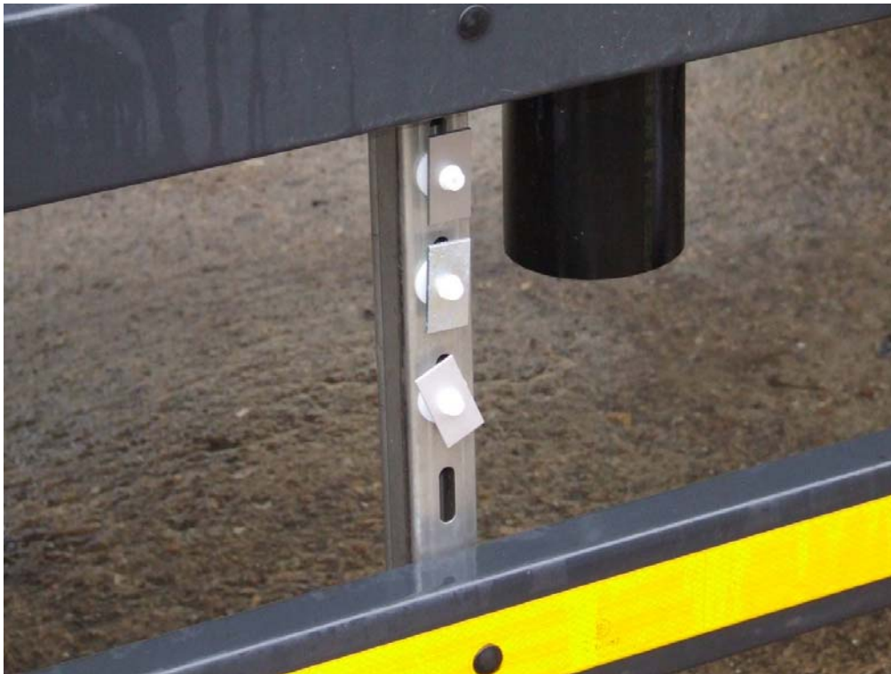
Plate 2-1 Side underrun bar support on Schmidt vehicle
