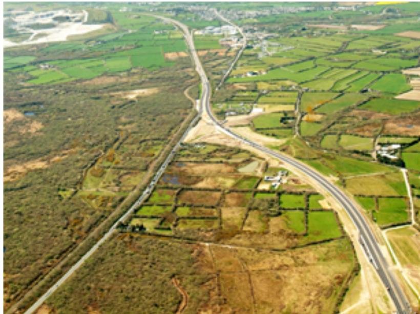
*This case study involved the construction of the A30 Bodmin-India Queens Improvement Scheme. The scheme upgraded this section of the A30 to dual carriageway and removed the previous height restrictions, easing congestion in the area. The project team undertook very effective resource efficiency measures to make the most of site won and locally available materials.*
