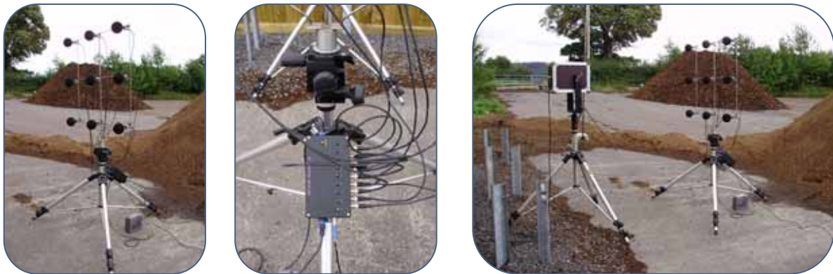
a) 9-microphone array b) Microphone switchbox c) Free-field measurement using 9-mic array
