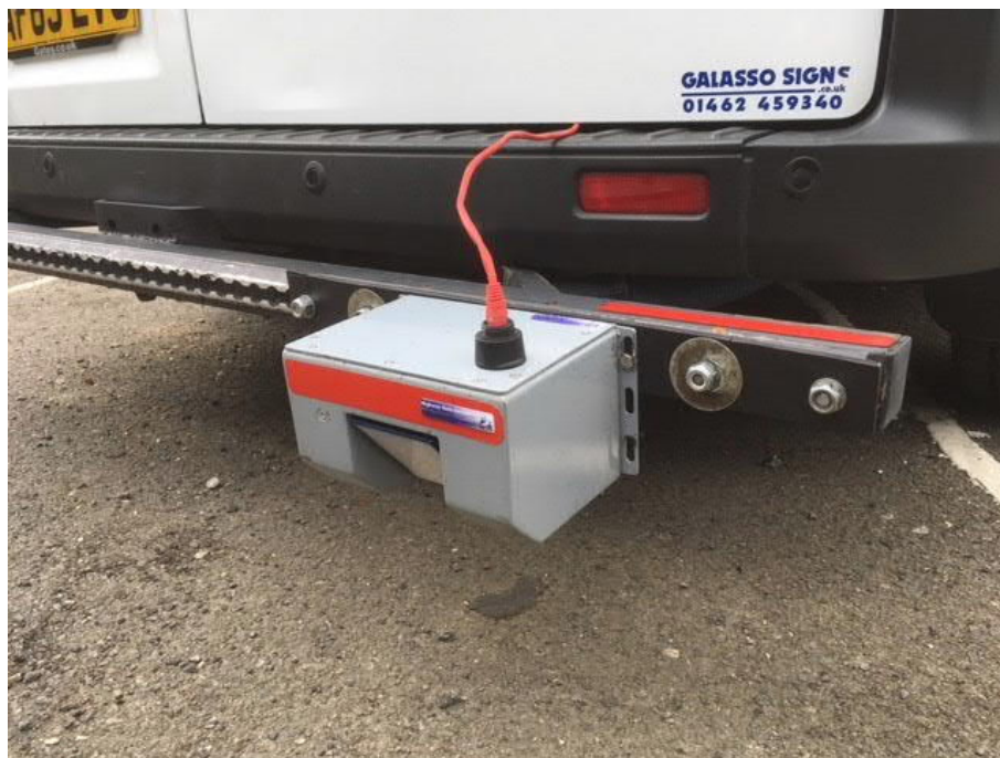
Figure 2 – Vehicle mounted Laser Straight Edge system (courtesy of MATtest Ltd)
