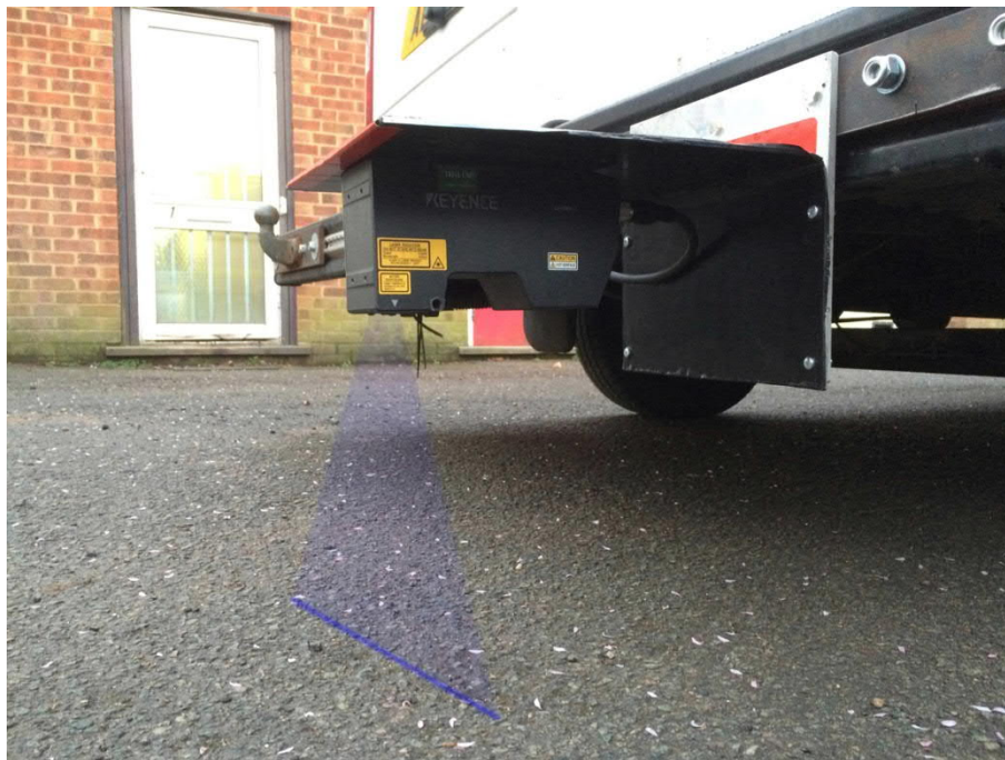
Figure 4 – MATtest vehicle mounted 3D-TD system (courtesy of MATtest Ltd).
