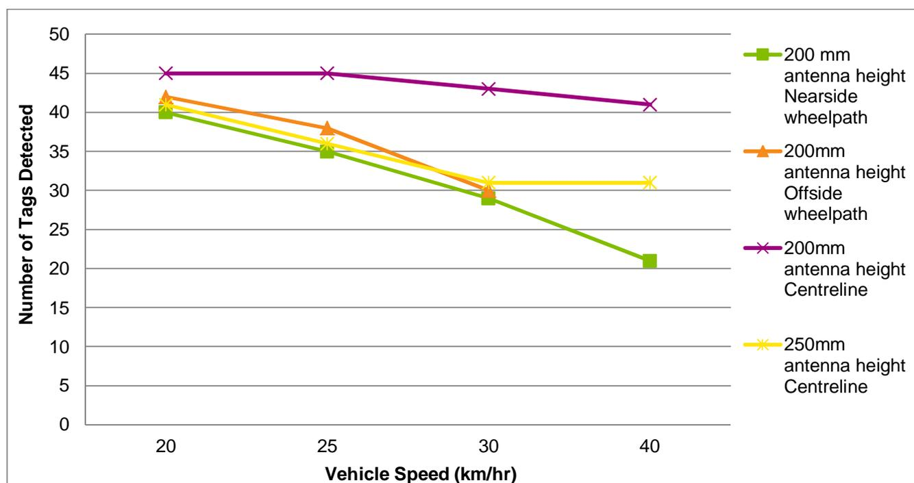
Figure 7: Trend Lines Showing Tags Detected (Vertical) Against Speed (Horizontal) at 200mm Antenna
