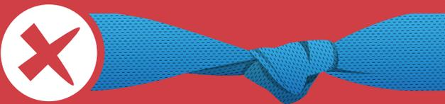
Never use a knot in any part of the strap that's under tension.
