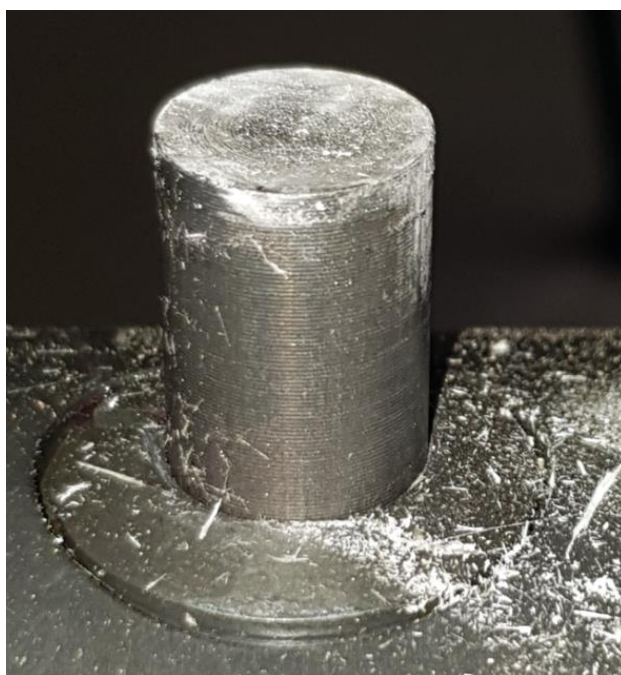
Figure 4 - Tubing Punch after use.
