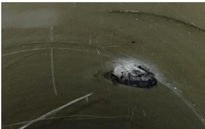
Figure 2 - Punched hole from inside of GRE lined tubing. The groove where some of the lining has unraveled can be seen.
