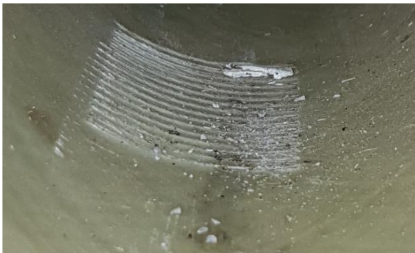
Figure 1 - Impression of tubing perforator slips on GRE after perforating
