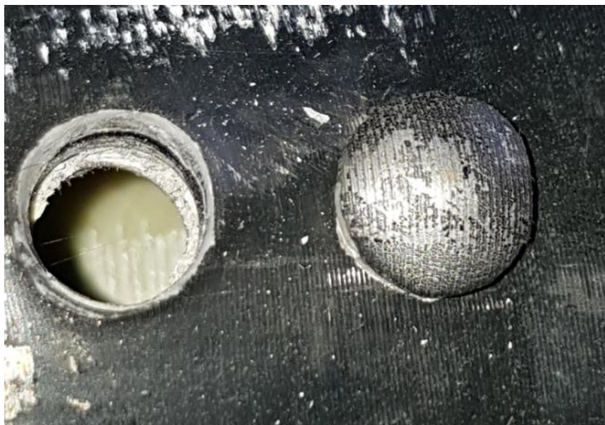
Figure 3 - Punched hole in the tubing from the outside with the punched section.
