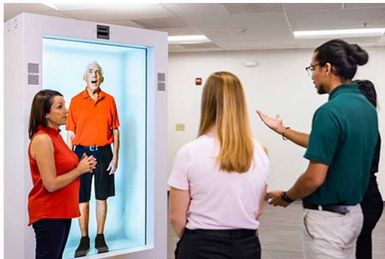
Figure 4. Human-sized 4K transparent LCD holoportation system in medical education at the University of Central Florida. Titled “Dr Hologram”, It will be used for patient simulation, allowing students to learn about a broader range of conditions (Campos, 2021).
