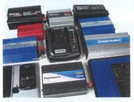
WE used a range of devices, including an iPhone 6, Blackberry 8800, iPad 4 and an HP Pavilion laptop to test these inverters. In addition, we used two pieces of garage kit in the shape of an 18V cordless drill charger and a 24-LED lead light. The best inverters could cope with all these devices being connected at the same time.
