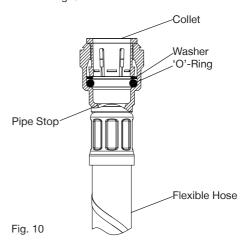
5. To release the joint, push pipe firmly into fitting, hold collet down and gently remove pipe. If the system has been filled with water care should be taken to isolate pump and towels used to absorb spilled water.
